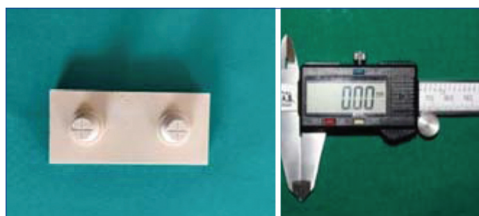
[Table/Fig-9]: Digital vernier caliper measuring inter abutment distance.
