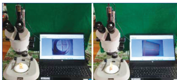
[Table/Fig-10]: Digital Stereomicroscope measuring diameter and height of the samples.
